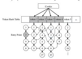
Fig. 2. URL redirection chain tracking process
